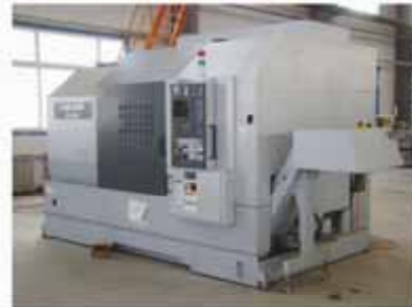
High precision CNC lathe can precisely manufacture thread and stress relief groove for pin and box tool joint.
