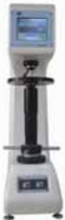
LC-200R Full-automatic Rockwell Hardness Tester ● Measure principle and method; sensor feedback electronic loading method/ linearly measure ● preloading: Newton: 29.42, 98.07 ● Main loading: Newton: 147.1, 294.2, 441.3, 588.4, 980.7, 1471 ● Time of Hold: 0-999# ● digital display, touchable LCD, sensor feedback electronic loading, accuracy up to 1.01HR
