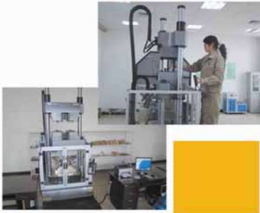
600DX Hydraulic pressure servo testing machine ● Loading Capacity: 600KN; Max test speed: 380mm/min; 600KN Max; 76mm/min; Returning Speed: 380mm/min; ● Max space of tensile test: 77 - 914mm; Compress test space: 32 - 565mm ● measure accuracy of loading; accuracy rate to readable numerical value: ± 0.5% ● Measure accuracy: ± 0.5% of readable numerical value;
